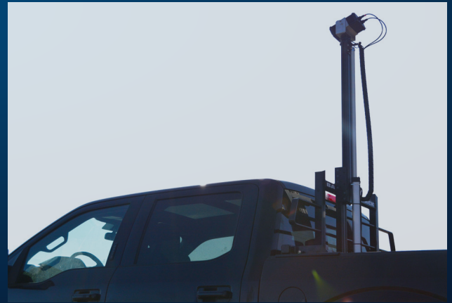
Two vehicle mounting configurations including roof rack for cars, vans and back rack for trucks.
