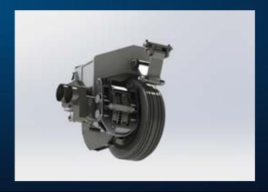
An aircraft anti-skid braking system (ASBS) and landing gear are mounted into the BAT<sup>TM</sup>.
